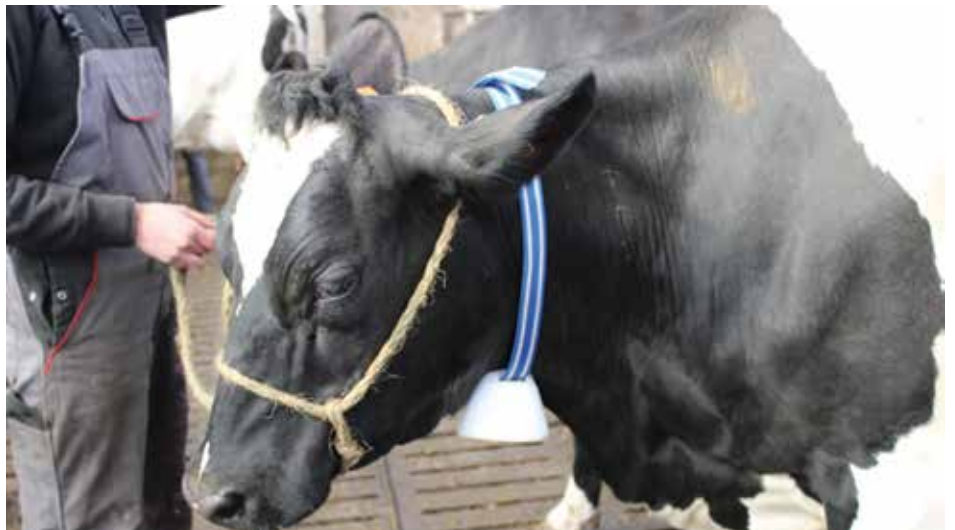
Figure 1: Collar with integrated accelerometers and temperature sensors, used in the MoniCow project.
